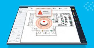
Samsung's built-in WIPS module in each AP provides excellent performance, accurately locating threats within 5 to 10 meters within a relatively large number of working sensors in the service space.
