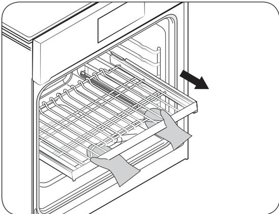
With the gliding rack closed, and the oven off and cool, grasp the rack, and frame and pull both forward to remove.
