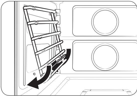
5. Swing the bottom of the rack support toward the oven-chamber wall.
