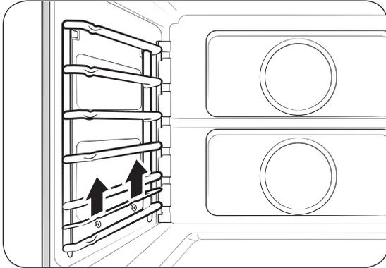
1. Grasp the bottom-center of the support, and lift.
