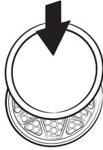
Centering the filter over the fan hole, carefully hook the metal clips (back of filter) over the metal bar across the hole. Do not scratch the oven's porcelain with the filter.
