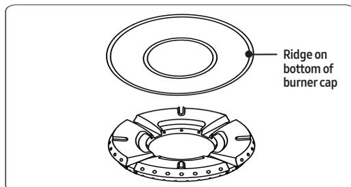
1. With power off and all surfaces cool, place the burner head so the locating tab goes into the keyed hole.
