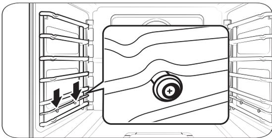
6. Pull the rack support down, making sure the two humps on the support bar rest upon the nuts attached to the oven-chamber wall.
