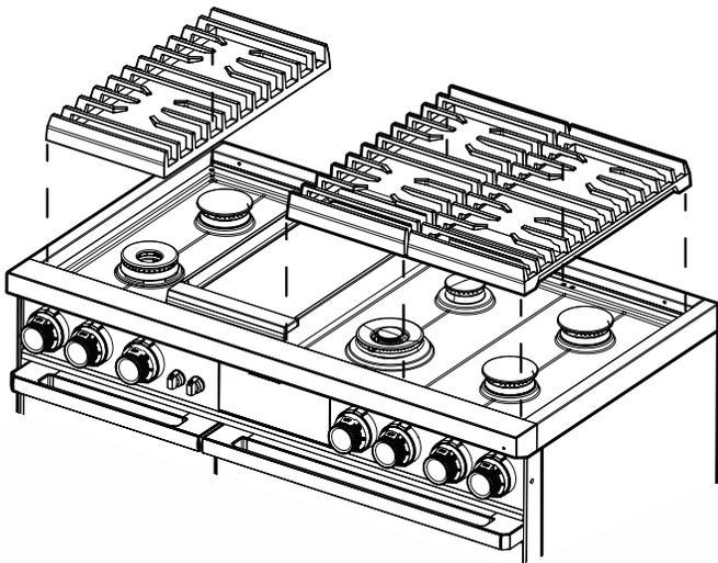
Check the underside of each grate for their proper position, then place the grates so their feet rest in the corresponding dimples. (Handle the heavy grates with care.)
