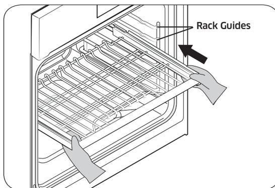
With the gliding rack slides retracted and the oven off, insert the rack between the guides until the rack reaches the back.
