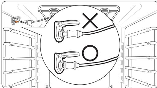
2. Insert the temp probe plug fully into the socket on the top side wall of the oven.
