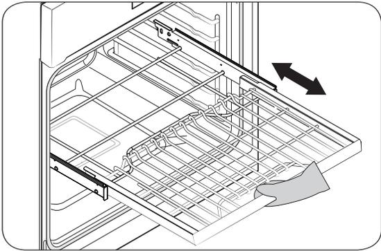
Grasp the handle to pull the gliding rack (left). Pulling by the frame may cause the rack to come off the guides, possibly harming the rack and the user. Wear oven mitts when handling the gliding rack during cooking.
