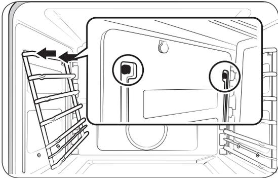
4. Insert the rack-support prongs into the holes near the top of the oven-chamber wall.
