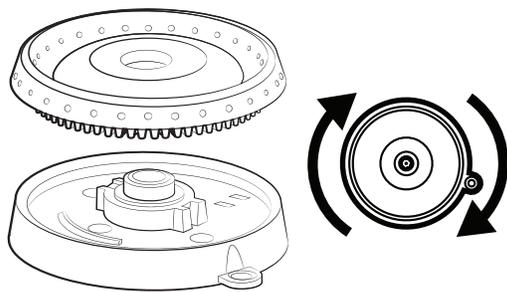
1. Put the burner heads on the burner bases as shown at left. (The bottom of the head fits inside the top of the base.)
