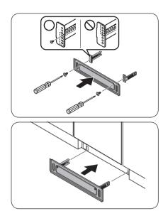
2. Attach the kickplate to the dishwasher using the kickplate brackets. Make sure the kickplate brackets are in the correct direction. See the figure for details.
