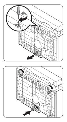
Turn the Torx T20 screwdriver counter clockwise as shown to remove the rear foot.
