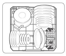
For more effective cleaning, load large items into the Storm Wash<sup>+</sup> area on the left side of the lower rack.
