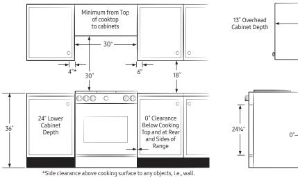
IMPORTANT: Consult with Installation Manual for detailed instructions before installing. All ranges must be installed with the Anti-Tip device that is included.
