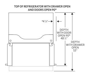
\*Allow 4¼" of clearance to enable doors to open 90° when installed next to a wall.
