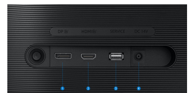
1 DisplayPort IN 2 HDMI IN 3 USB/SERVICE 4 DC14V
