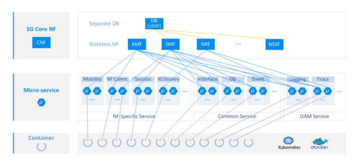
Figure 4-3. Samsung 5G Core: Cloud Native Architecture
