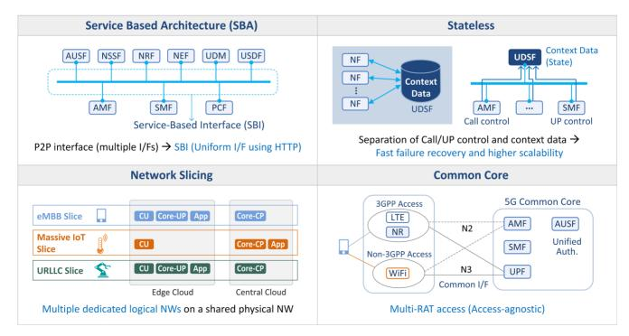
Figure 2-1. 5G Core Network Design Principle
