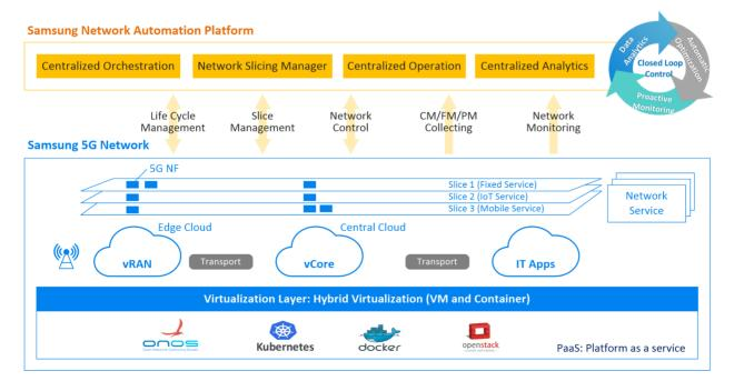
Figure 4-1. Samsung 5G Network Automation Architecture
